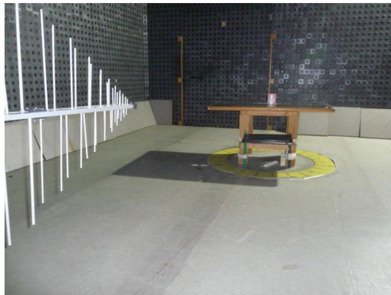
Photograph 8.1.1 Setup for radiated emission measurements
