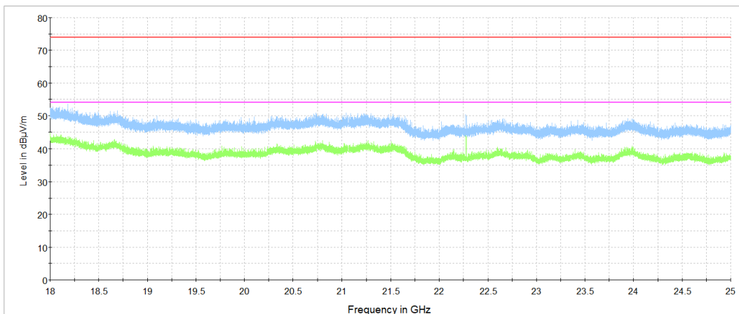
Plot 7.3.50 Radiated emission measurements from 18000 to 25000 MHz at the high carrier frequency 2480 MHz Antenna 2
