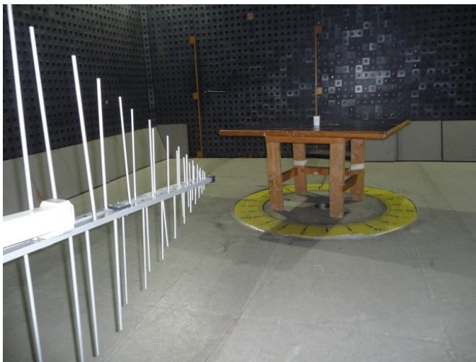
Photograph 8.1.1 Setup for radiated emission measurements
