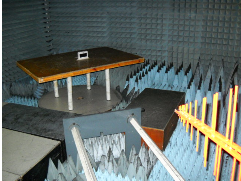
Photograph No.4 Setup for OBW measurements in the anechoic chamber in 30 – 1000 MHz range
