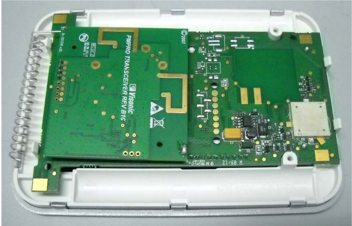
Photograph No.1 Touch screen keyprox internal view
