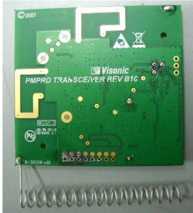
Photograph No.5 RFD module
