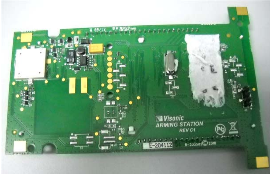
Photograph No.4 Main PCB front view without RF module
