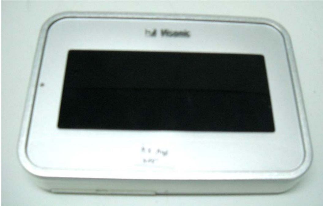
Photograph No.1 Touch screen keyprox general view
