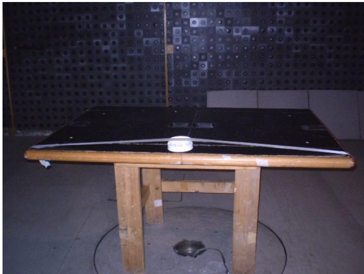
Photograph 7.5.3 Setup for final radiated emission measurements, EUT close view
