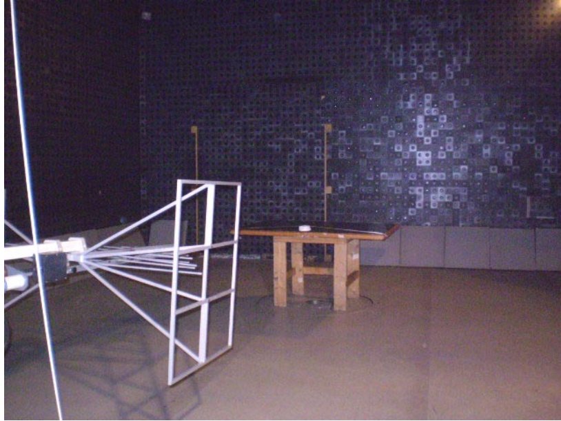
Photograph No.6 Setup for radiated emission measurements in the anechoic chamber in 30 – 1000 MHz range
