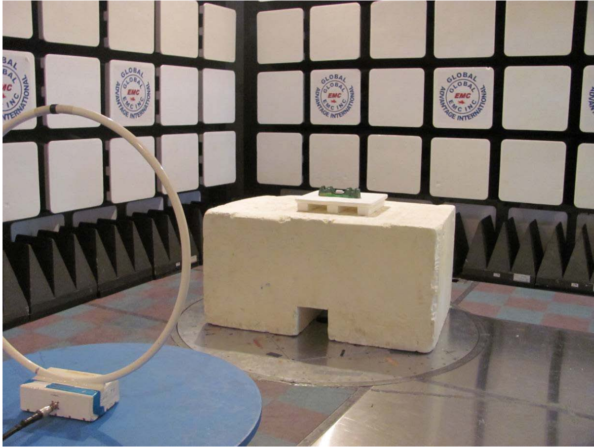
Figure 4: Radiated emission setup – photo 4
