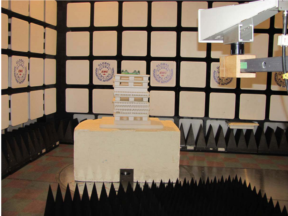
Figure 2: Radiated emission setup – photo 2
