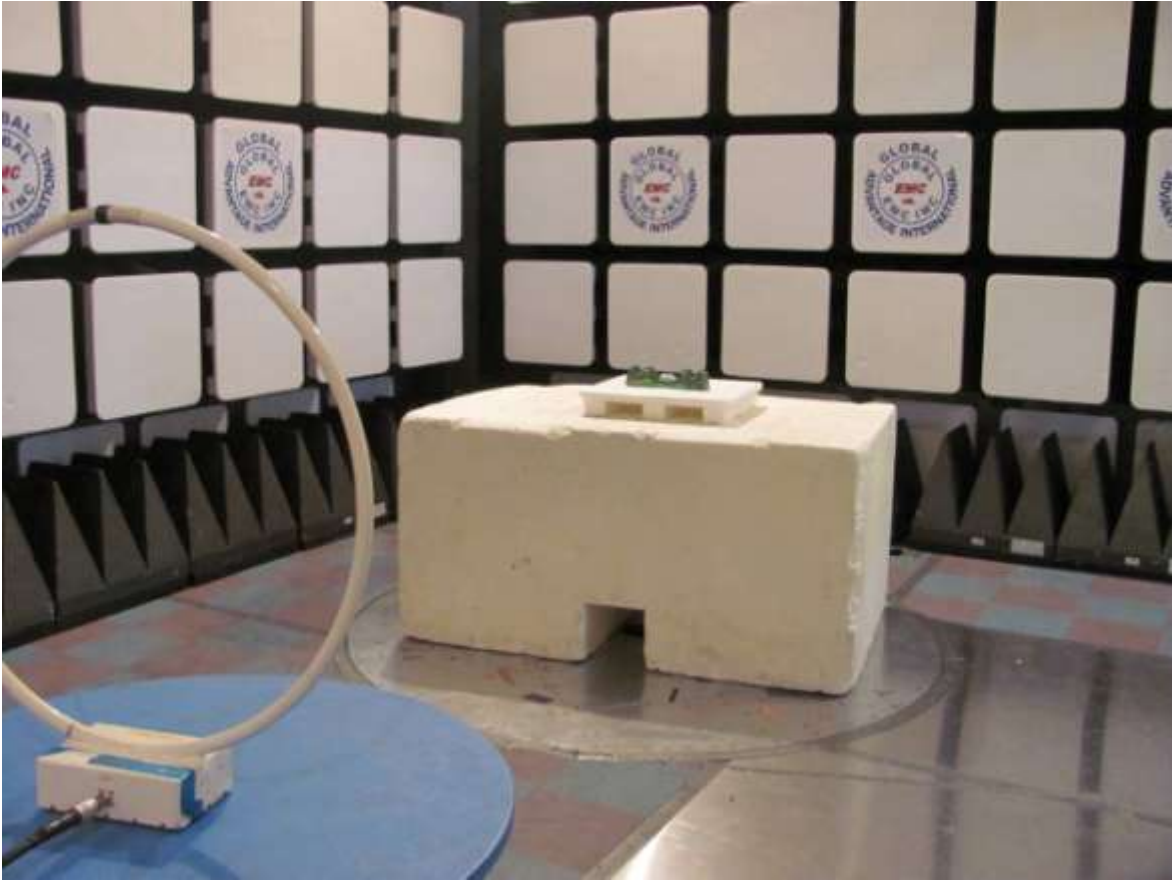
Figure 4: Radiated emission setup – photo 4
