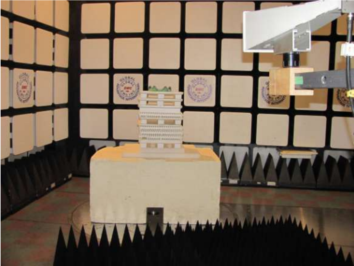
Figure 2: Radiated emission setup – photo 2
