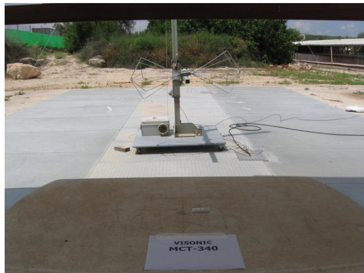
Figure 5. Radiated Emission Test
