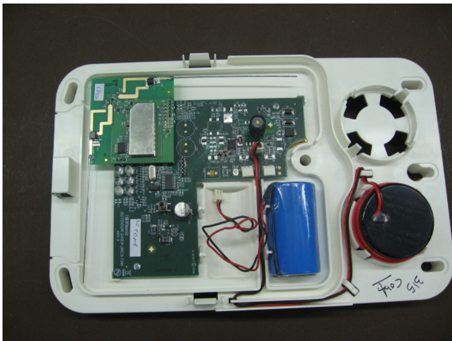
Figure 2: Circuit boards, battery, and alarm
