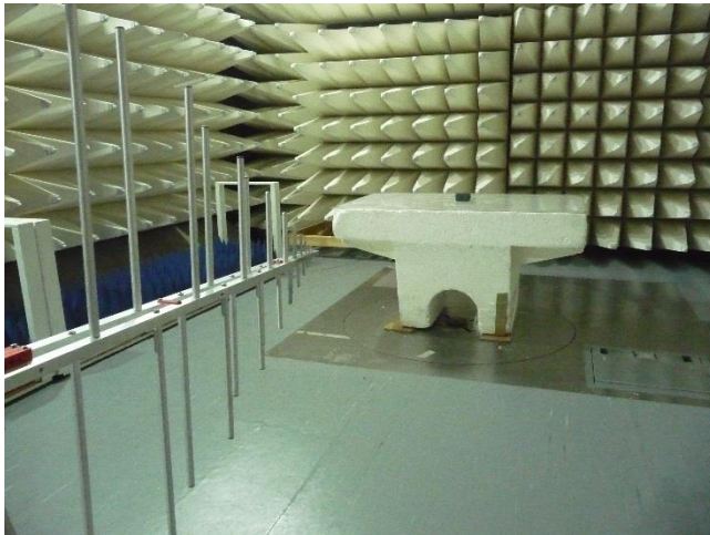
Photograph 8.1.1 Setup for radiated emission measurements
