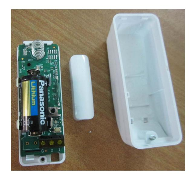
Photograph No.2 MC-309 PG2 magnetic contact internal view without battery
