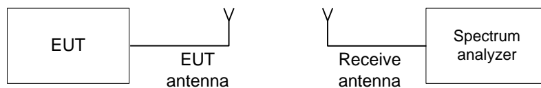
Figure 7.3.1 Hopping frequencies test setup
