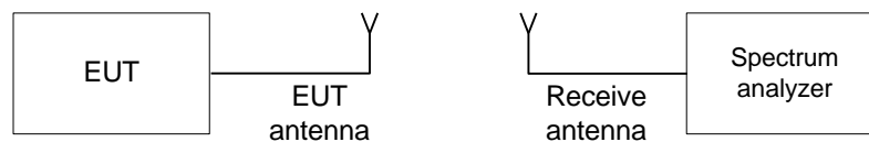
Figure 7.7.1 Band edge emission test setup
