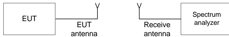
Figure 7.1.1 The 20 dB bandwidth test setup
