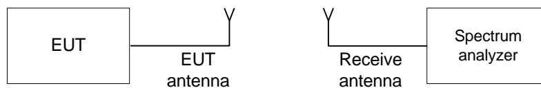
Figure 7.3.1 Hopping frequencies test setup
