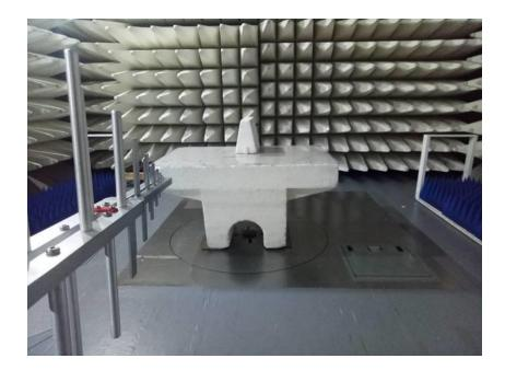
Photograph No.5 Setup for field strength measurements in anechoic chamber above 1 GHz
