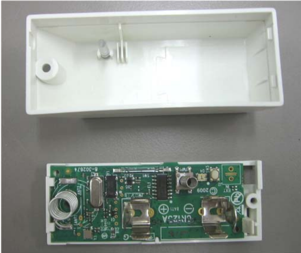
Photograph No.1 Magnetic contact device internal view
