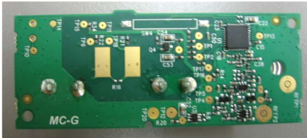
Photograph No.3 Magnetic contact device PCB rear side view
