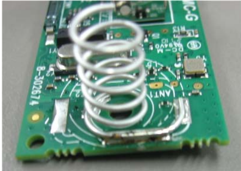
Photograph No.4 Magnetic contact device antenna
