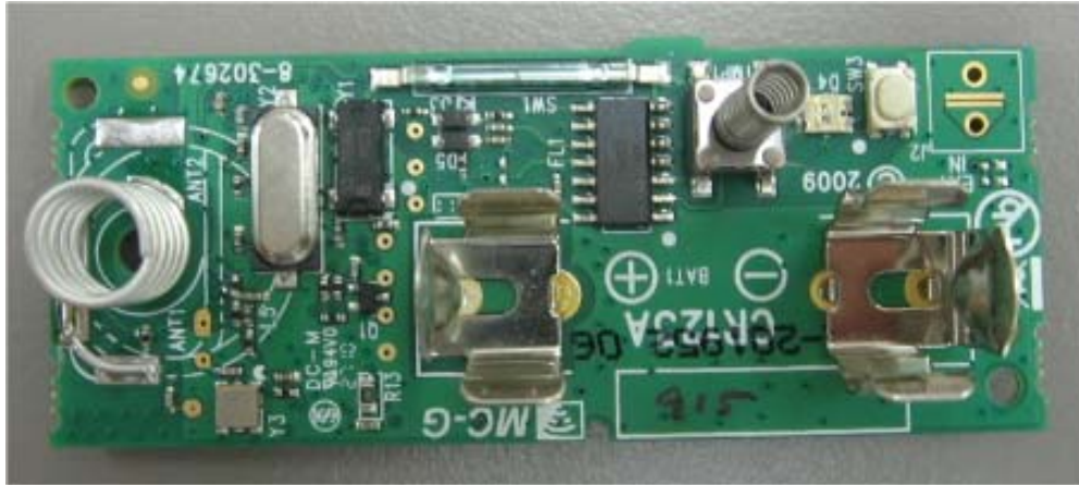
Photograph No.2 Magnetic contact device PCB front view
