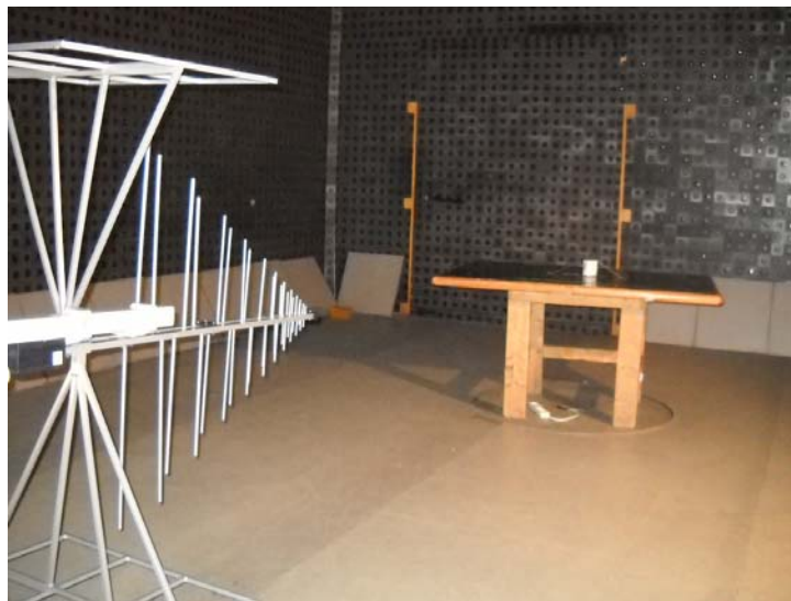
Photograph 8.1.1 Setup for radiated emission measurements
