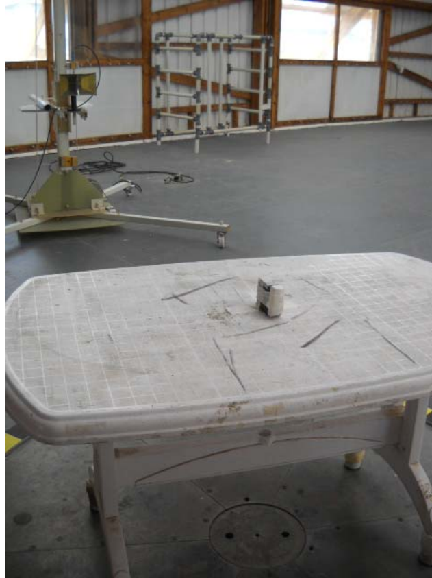
Photograph No.4 Setup for spurious emission field strength measurements at the OATS above 1000 MHz range
