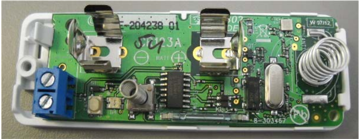
Photograph No.1 Magnetic contact device internal view
