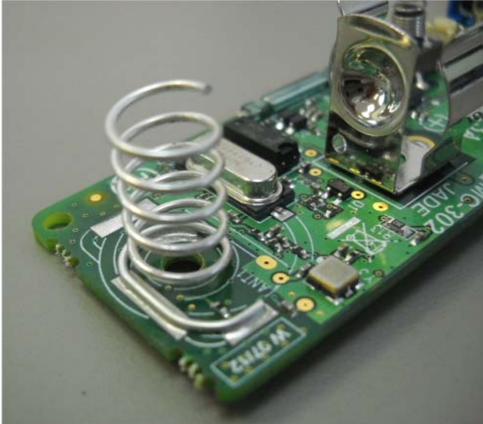
Photograph No.3 Magnetic contact device antenna
