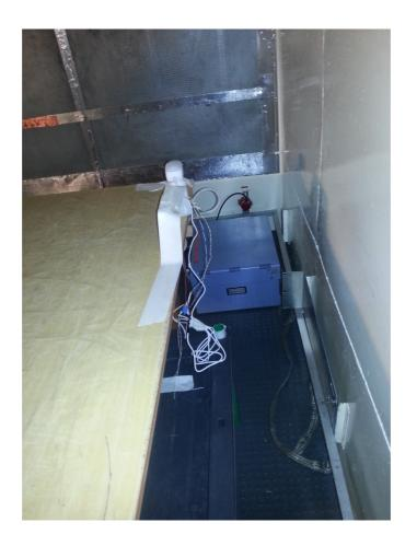
Photograph No.8 Setup for conducted emission measurements on the AC power lines
