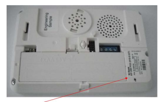
Label with FCC ID:WP3KP250PG2 and IC:1467C-KP250PG2 will be located at the rear side panel of the keypad. The statement according to FCC part 15 §15.19(a)(3) is placed in Installer's Guide, page 88 (Application exhibit KP-250\_UserMan).
