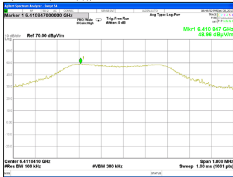
Plot 7.7.52 Radiated emission measurements at the seventh harmonic of mid carrier frequency
