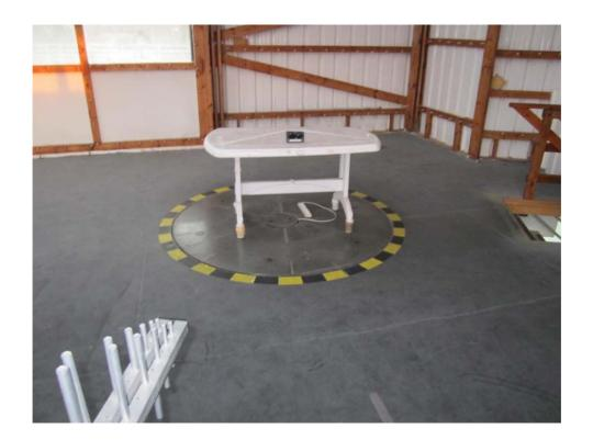
${\bf Photograph~No.5}$  Setup for carrier field strength measurements at the OATS in 30 – 1000 MHz range, EUT close view
