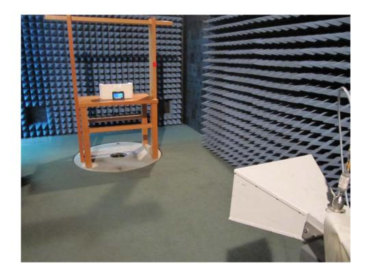
${\bf Photograph~No.4}\\ {\bf Setup~for~carrier~field~strength~measurements~at~the~OATS~in~30-1000~MHz~range}$
