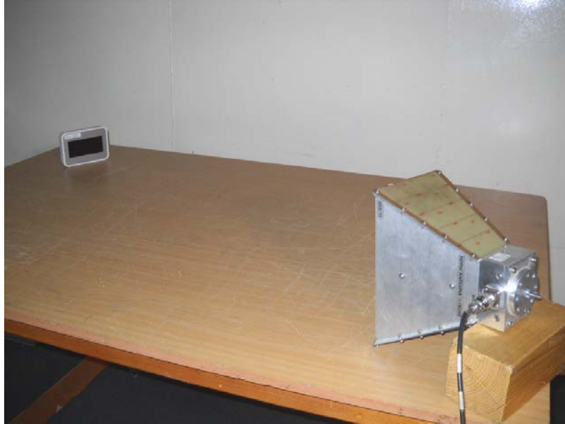
Photograph No.5 Setup for band edge emission and hopping parameters measurements in the shielded room
