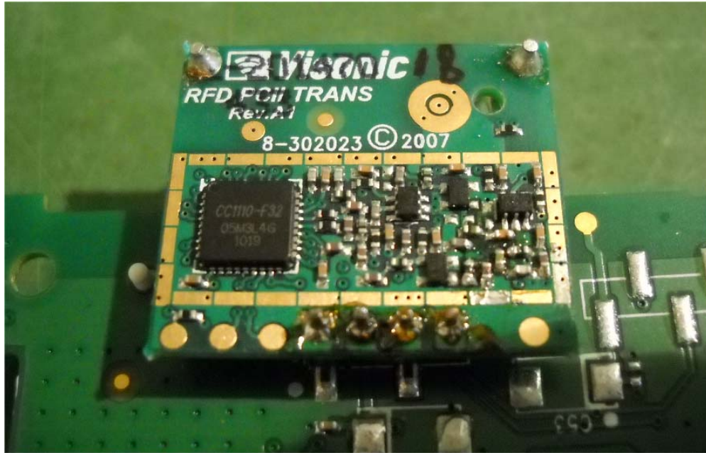
Photograph No.5 RFD module
