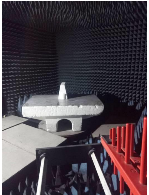
Photograph 8.1.2 Setup for final radiated emission measurements, EUT cabling
