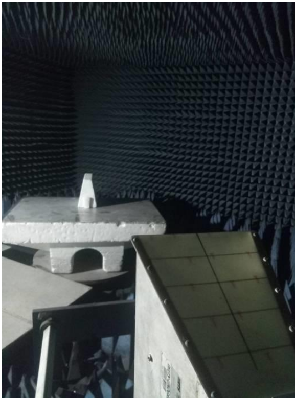
Photograph 8.1.2 Setup for final radiated emission measurements, EUT cabling
