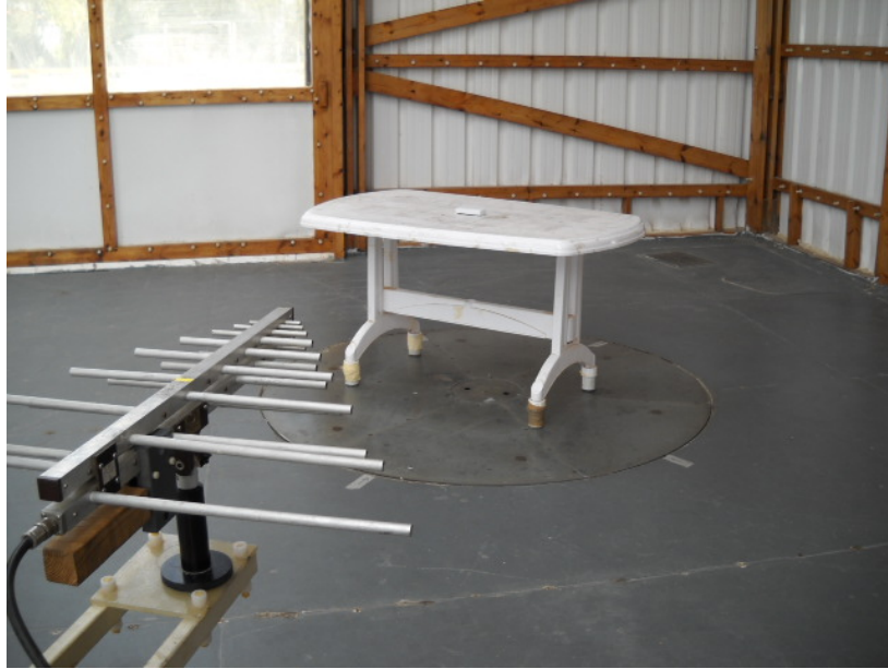
Photograph No.4 Setup for OBW, carrier field strength, spurious emission field strength measurements at the OATS in 30 – 1000 MHz range
