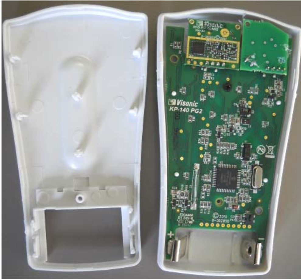
Photograph No.1 Remote keypad internal view
