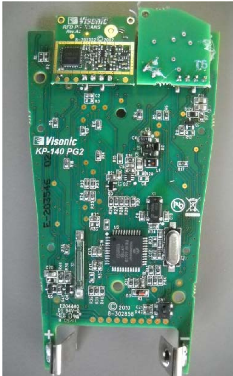
Photograph No.3 Main board with RFD and RFID modules
