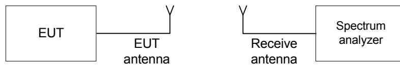
Figure 7.1.1 The 20 dB bandwidth test setup
