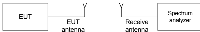
Figure 7.2.1 Carrier frequency separation test setup
