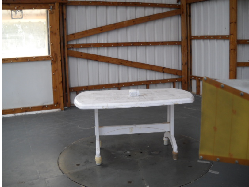
Photograph No.5 Setup for spurious emission field strength measurements at the OATS above 1000 MHz range
