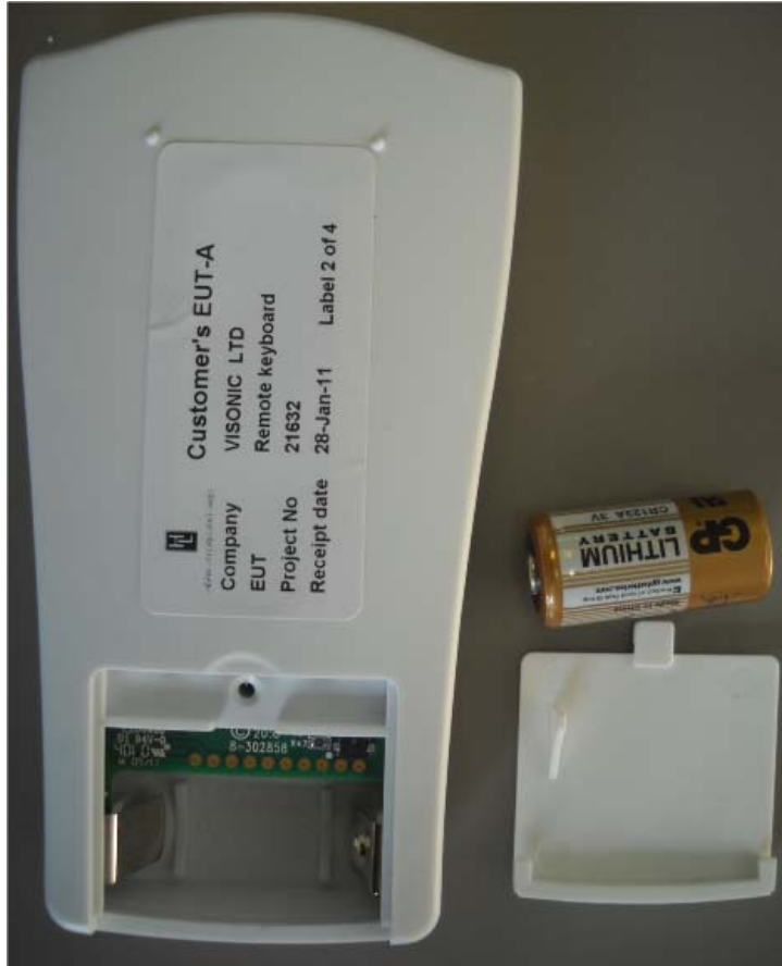
Photograph No.4 Remote keypad rear side with cover and battery removed
