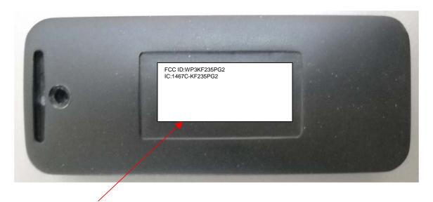
Label with FCC ID:WP3KF235PG2 and IC:1467C-KF235PG2 will be located at the rear side panel.
