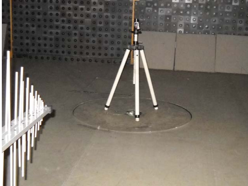
Photograph No.2 Setup for carrier, OBW, hopping frequencies and spurious emission field strength measurements in the anechoic chamber in 30 – 1000 MHz range
