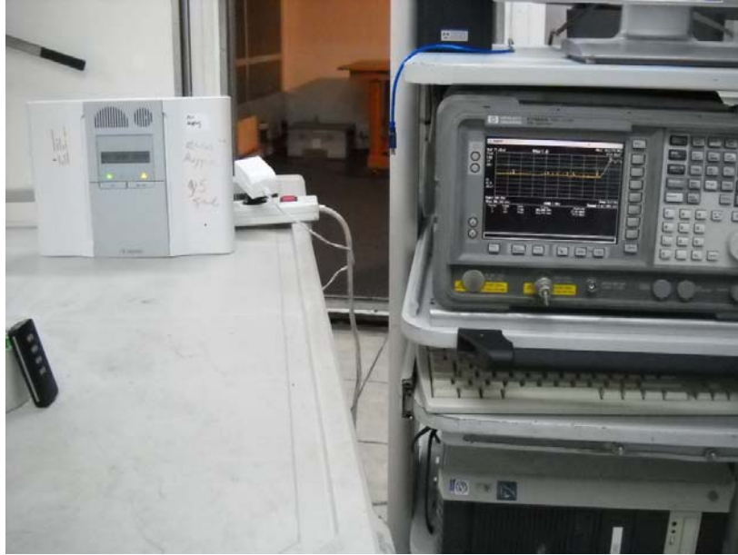
Photograph No.5 Setup for band edge emission measurements
