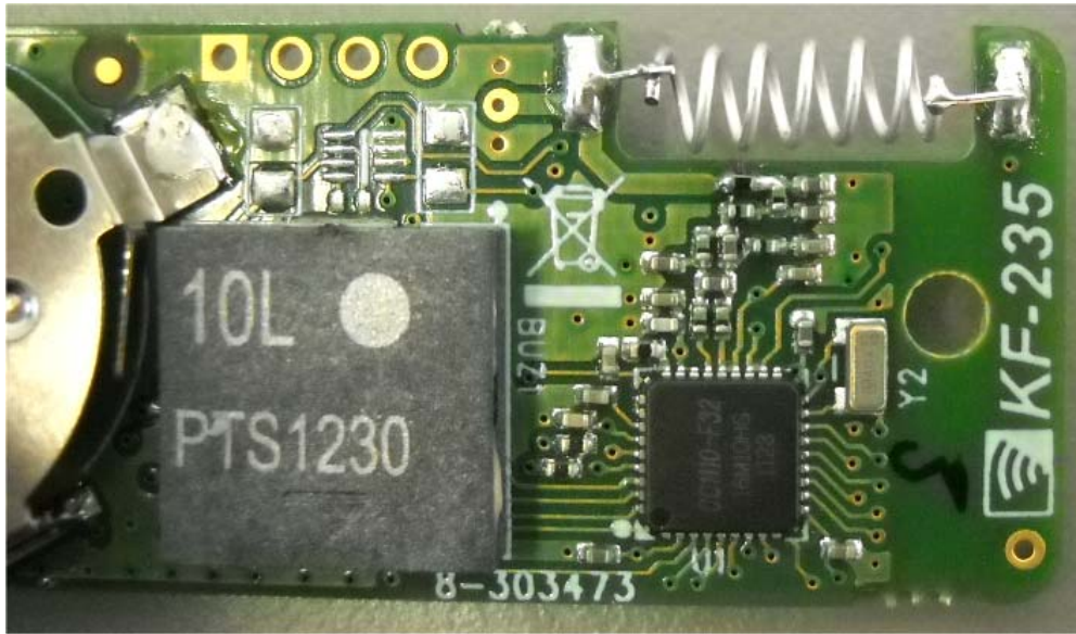
Photograph No.4 Wireless 2-way keyfob KF-235 PG2 antenna
