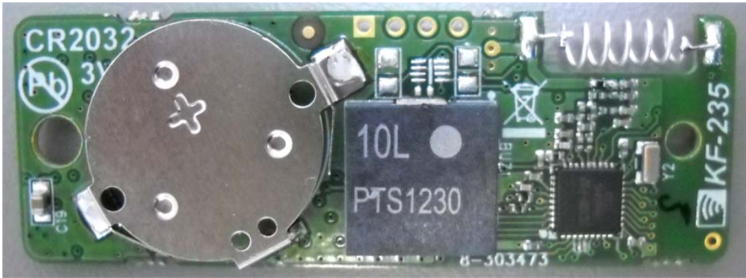
Photograph No.2 Keyfob PCB front view
