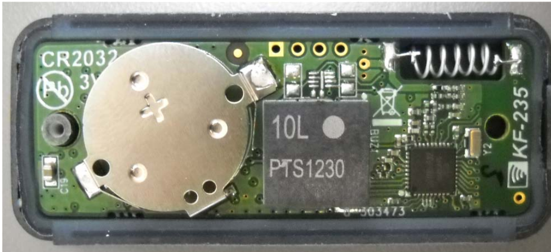
Photograph No.1 Wireless 2-way keyfob KF-235 PG2 internal view
