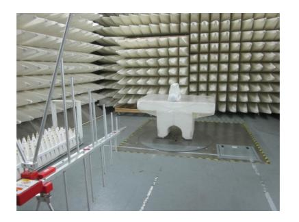
Photograph No.1 Setup for carrier field strength measurements for EUT in X-axis position
