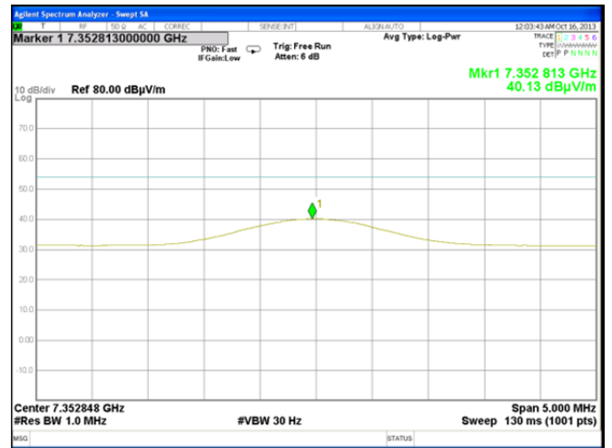
Plot 7.7.40 Radiated emission measurements at the ninth harmonic of low carrier frequency
