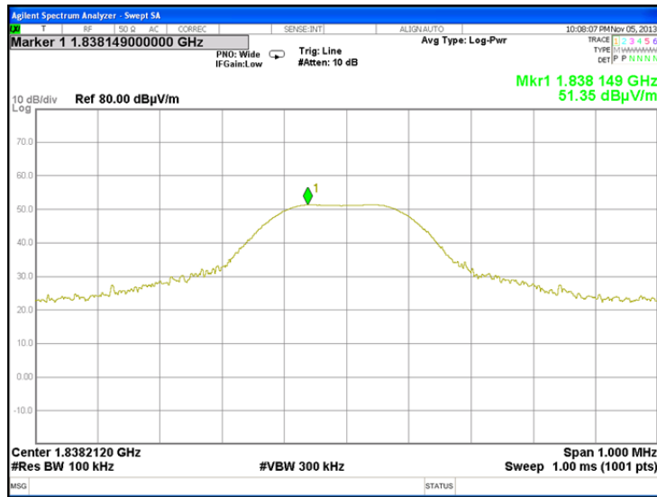
Plot 7.7.22 Radiated emission measurements at the third harmonic of low carrier frequency
