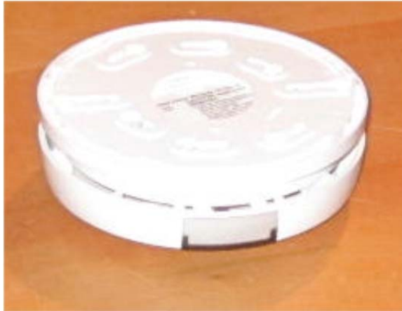
Photograph 6.4.1 EUT in X-axis orthogonal position
