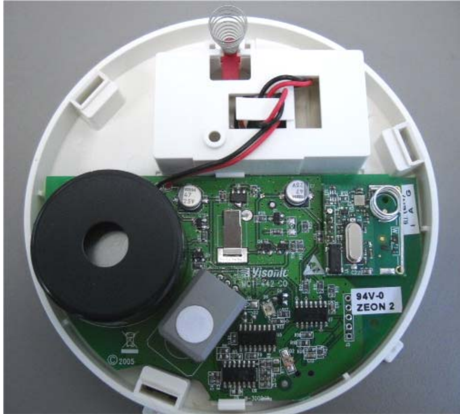
Photograph No.1 CO gas detector internal view
