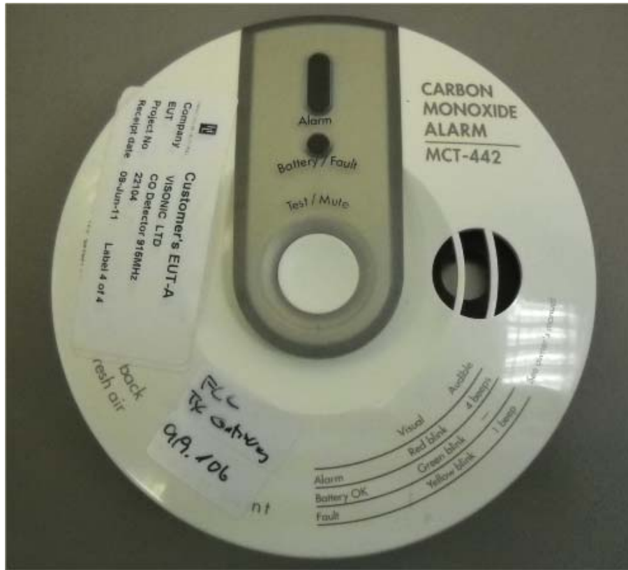
Photograph No.1 CO gas detector front view
