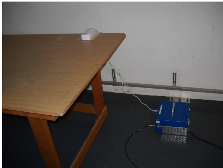
Photograph 8.1.1 Setup for conducted emission measurements at AC mains input port
