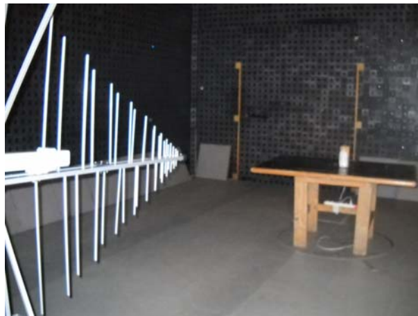
Photograph 8.2.1 Setup for radiated emission measurements
