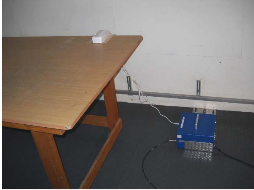
Photograph No.6 Conducted emissions on AC power lines test setup
