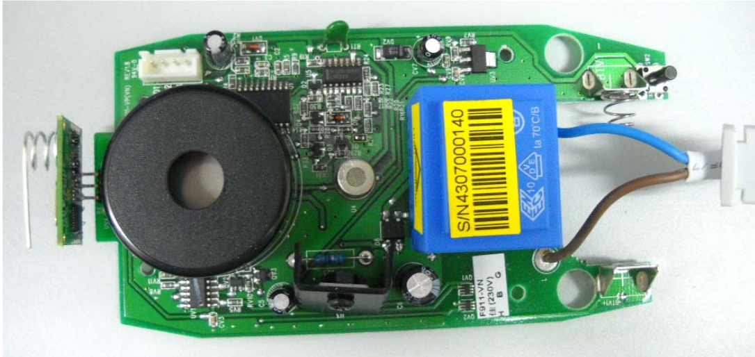
Photograph No.2 Main PCB with RFD module front view
