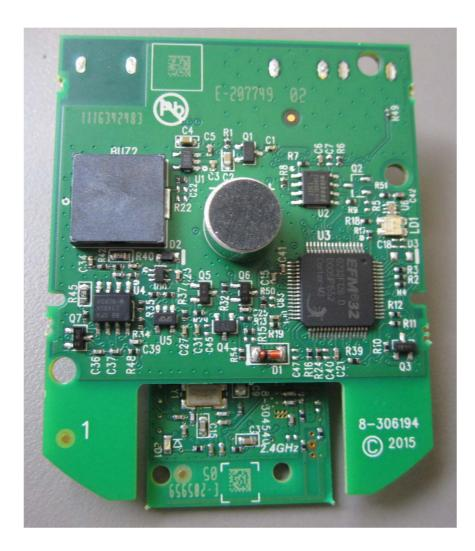
Photograph No.4 GB-540 glass break PCB rear side view
