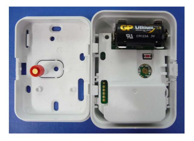
Photograph No.1 GB-540 glass break detector internal view
