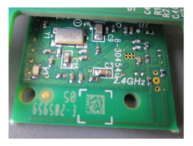
Photograph No.6 GB-540 detector RF board second side view
