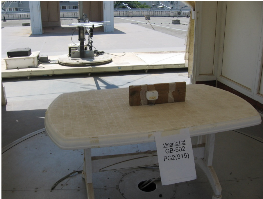
Figure 6. Radiated Emission Test – Wall Mounted
