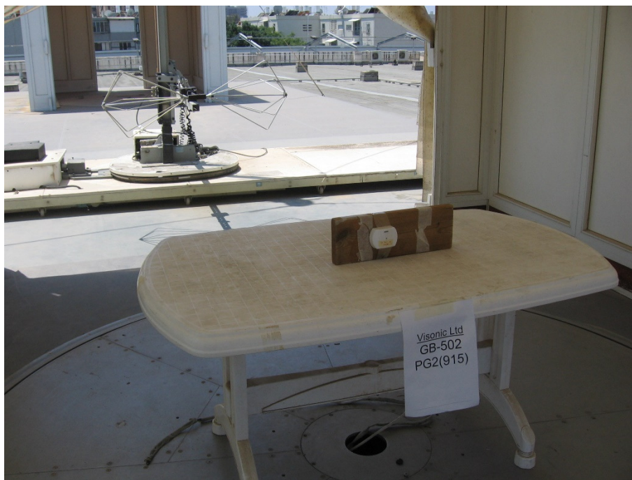
Figure 7. Radiated Emission Test – Wall Mounted
