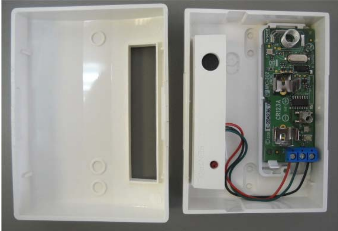
Photograph No.1 Wireless glass-break detector GB-501 PG2 internal view
