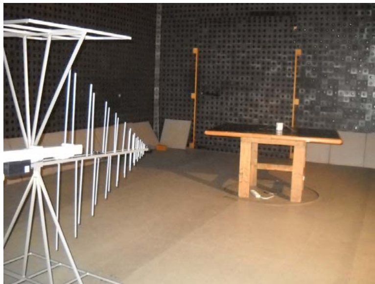
Photograph 8.1.1 Setup for radiated emission measurements
