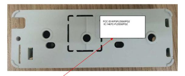
Label with FCC ID:WP3FLD550PG2 and IC:1467C-FLD550PG2 is located at the rear side panel. The statement according to FCC part 15 §15.19(a)(3) is placed in User's Guide, page 3 (Application exhibit User\_manual\_23018).
