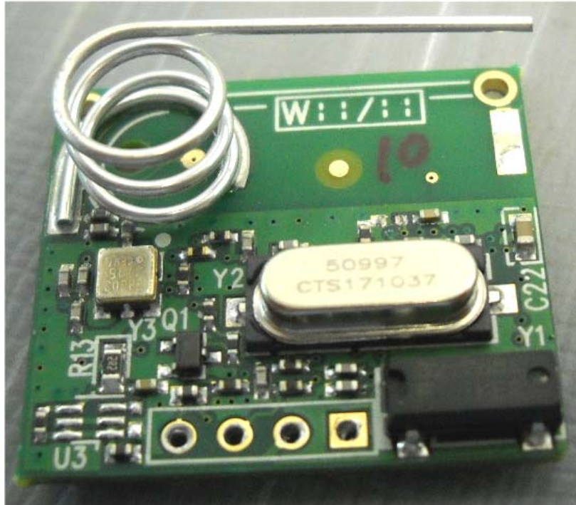
Photograph No.4 RFD module
