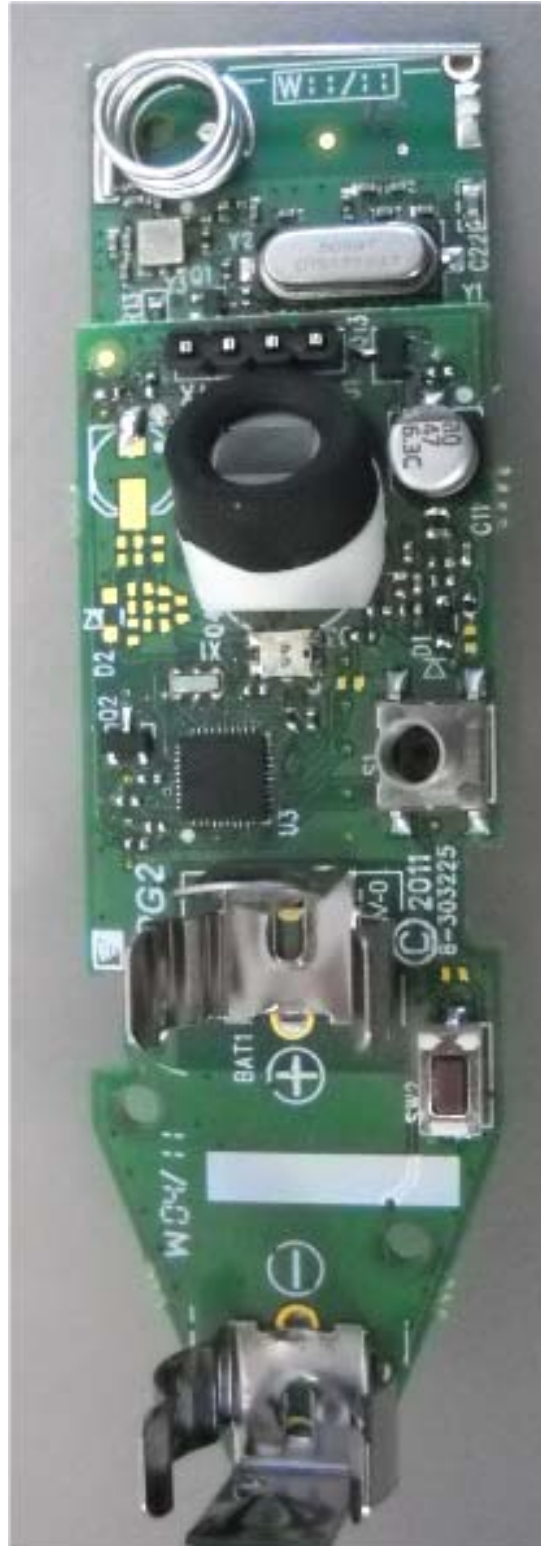
Photograph No.2 Main PCB with RFD module front view
