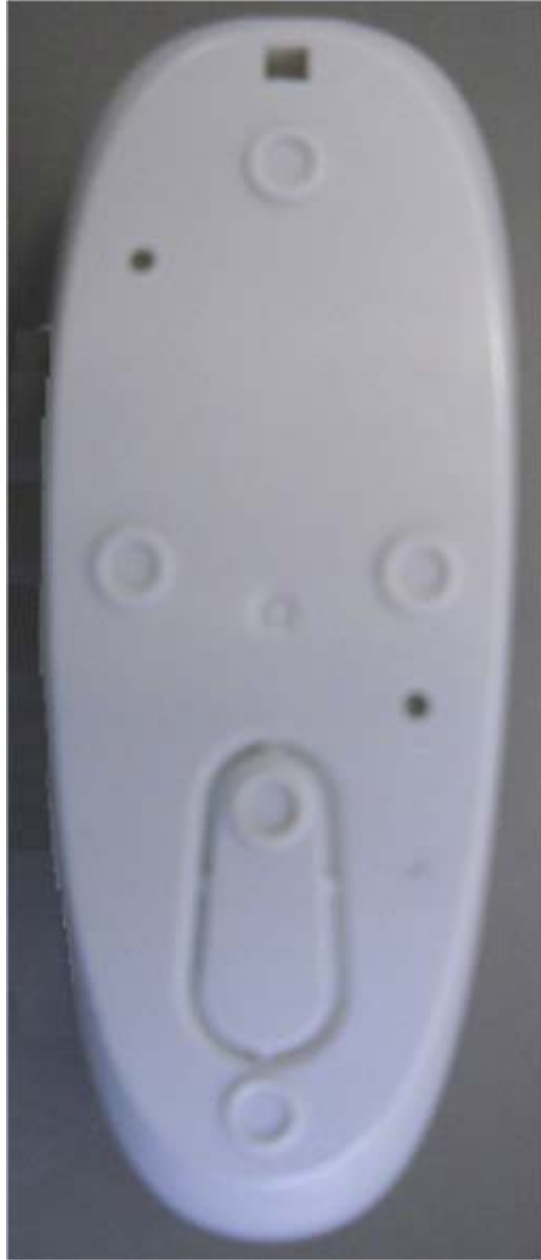
Photograph No.2 “CLIP PG2” PIR detector rear side view
