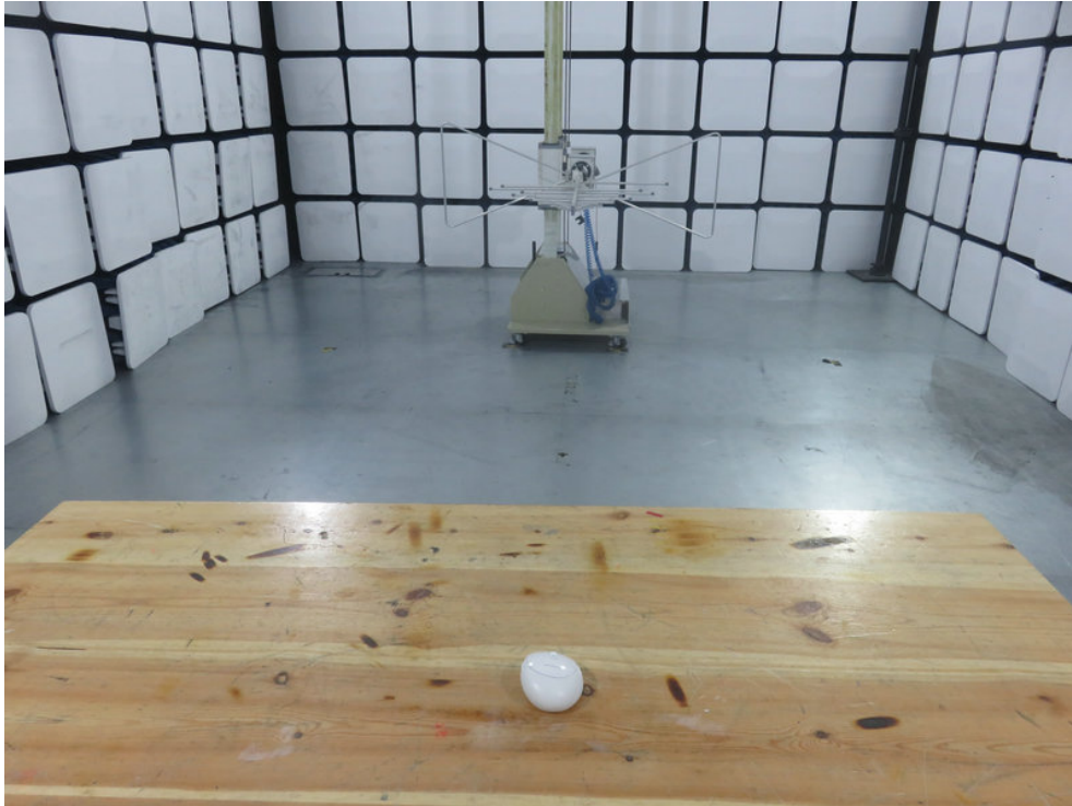
Photo of Radiation Emission Test
